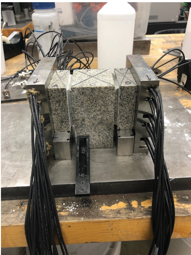
A rock sample is sandwiched between sensor-equipped steel plates prior to testing.
