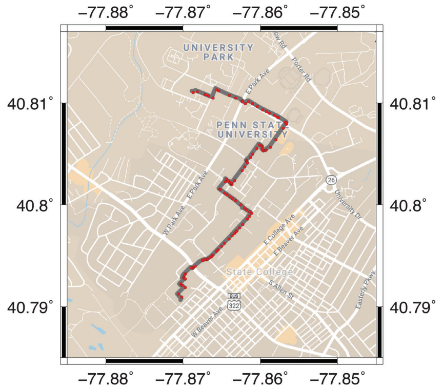
Penn State fiber-optic distributed acoustic sensing (DAS) array map. Red dots indicate our tap test locations.
