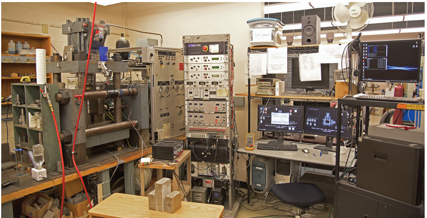
The biaxial earthquake machine in the Rock and Sediment Mechanics Laboratory, uses steel blocks driven by horizontal and vertical hydraulic pistons to simulate conditions on natural faults.
