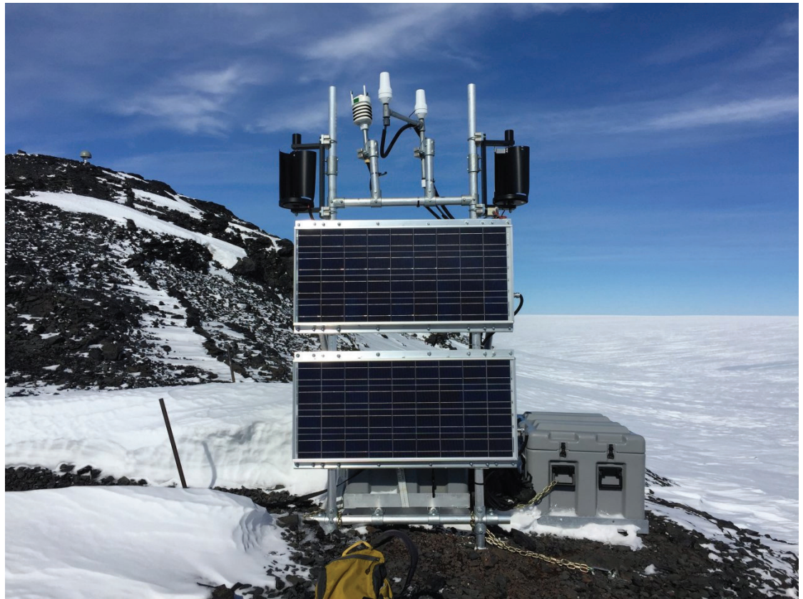
Close up photo of Polar Earth Observing Network monitoring station that collects GPS and seismic measurements to understand ice sheet behavior. Credit: POLENET
