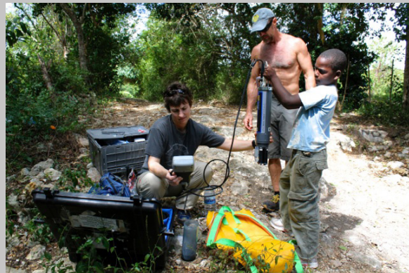
Jenn Macalady (left) and a local volunteer prepare a water chemistry data logger that will be carried by cave diver Kenneth Broad (right). The geochemical data will shed light on microbial iron and nitrogen cycling in the terrestrial subsurface. Photo credit Dominican Republic Speleological Society. Photo credit: Jenn Macalady
